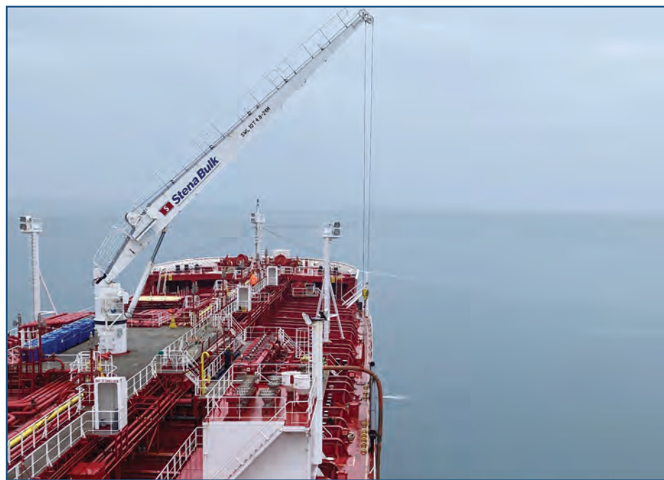
The Stena Imperative is secured in the in Multi-Point Mooring with hose attached and ready to discharge cargo.
